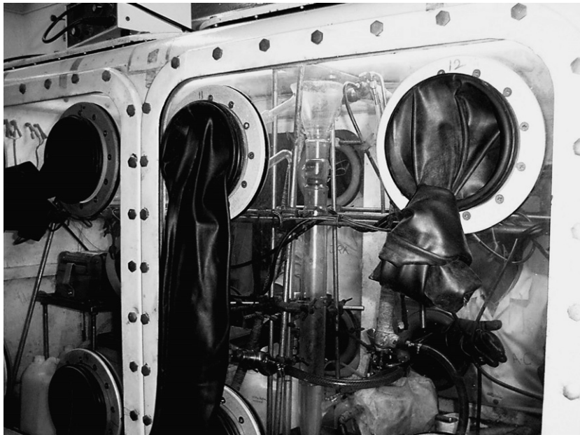
Fig. 2. Gelation assembly used for the preparation of (U,Pu)O 2 microspheres.
